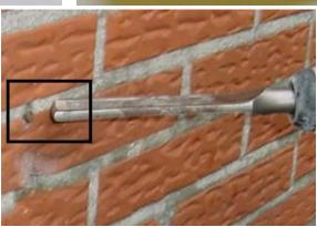
In some cases it could be possible that there was no optimal bonding between the soldering process of the teeth and the chisel metal. Through the mechanical vibration of the chipping hammer (machine) the teeth then spontaneously fall out of the chisel.
